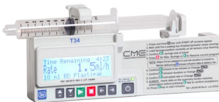
Fig. 3. T34 syringe pump, set in ml/hr, with additional alarms including: syringe removed, low battery, nearly empty and occlusion alarm.
