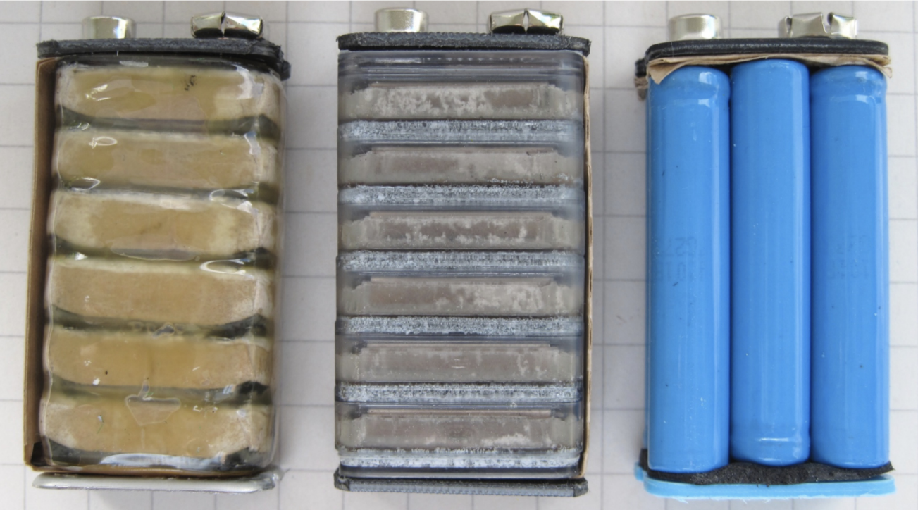
Internal cell structure varies from battery to battery type courtesy of wikipedia
